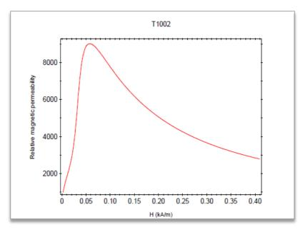
Figure 1: Permeability curve of a grade of Transil
