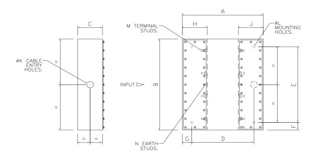
Masking: Rear stainless-steel finish. Input piercing masked to 60mm.
